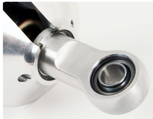
Figure 13 - Snap Ring Installed
