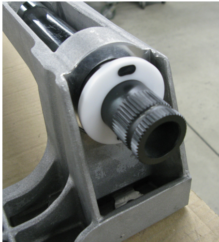
Figure 8: Installing the Delrin Bushing
