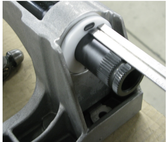
Figure 9: Measuring the Anti-Roll Bar
