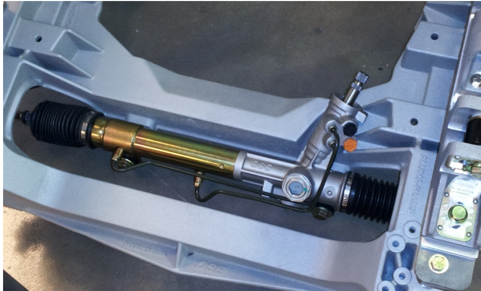
Figure 7: Installed Rack and Pinion
