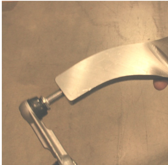
Figure 11: Pre-assemble the Anti-Roll Bar End Links
