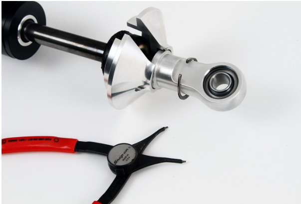
Figure 12 - Removing the Snap Ring
