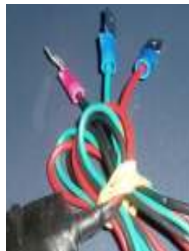
Lead wires on LED flasher module.
