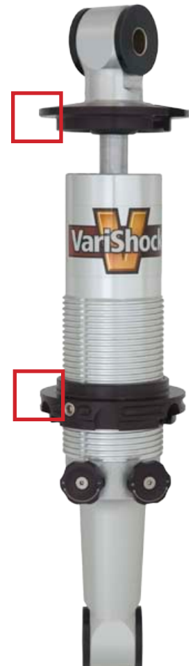
Hook the tape measure against the spring at the upper spring seat slot.
