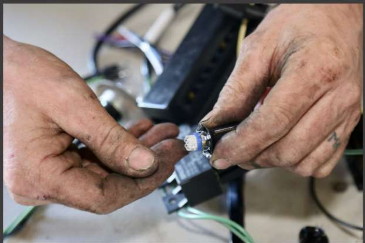
Some of the instrument panel lights were replaced with blue LEDs from Scott Drake. The alternator and oil warning lights were fitted with replacement incandescent bulbs because they are behind red lenses on the instrument panel. Also, the high-beam bulb was left incandescent because it's behind a green lens.
