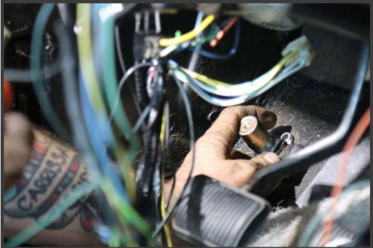
The new Scott Drake dimmer switch is installed.
