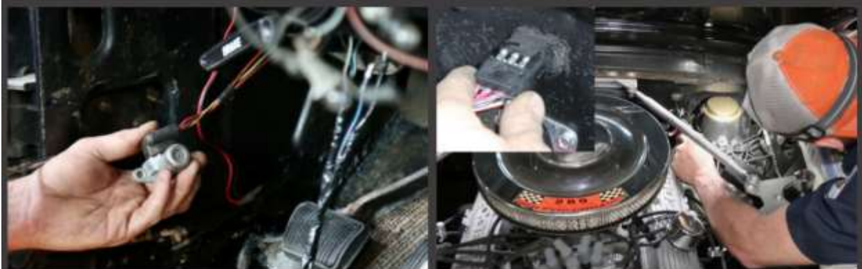
The high beams weren't working, so the floor-mounted dimmer switch was removed and disconnected. Note that the left sill plate and kick panel have already been removed, which also exposed the connection for the taillight harness down in the rocker area. The firewall plug leading to the engine harness is disconnected.
