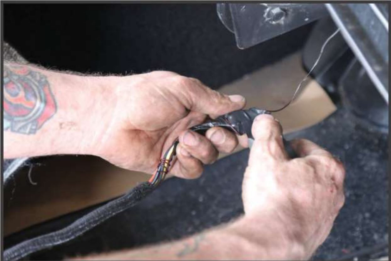
Here's the new Scott Drake harness ready to be pulled with the snake from the trunk. Once positioned, the taillights were easily connected along with the wires to the interior lamps on each side.
