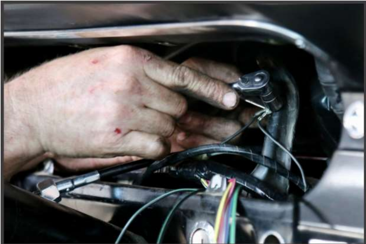
The ground wires are secured with a new fastener.
