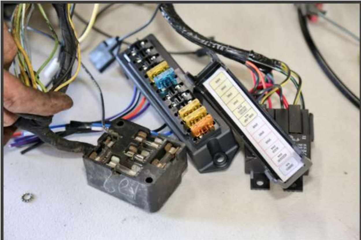
Here's a side-by-side view of the factory fuse box and the upgraded ATC fuse block in the Scott Drake harness.
