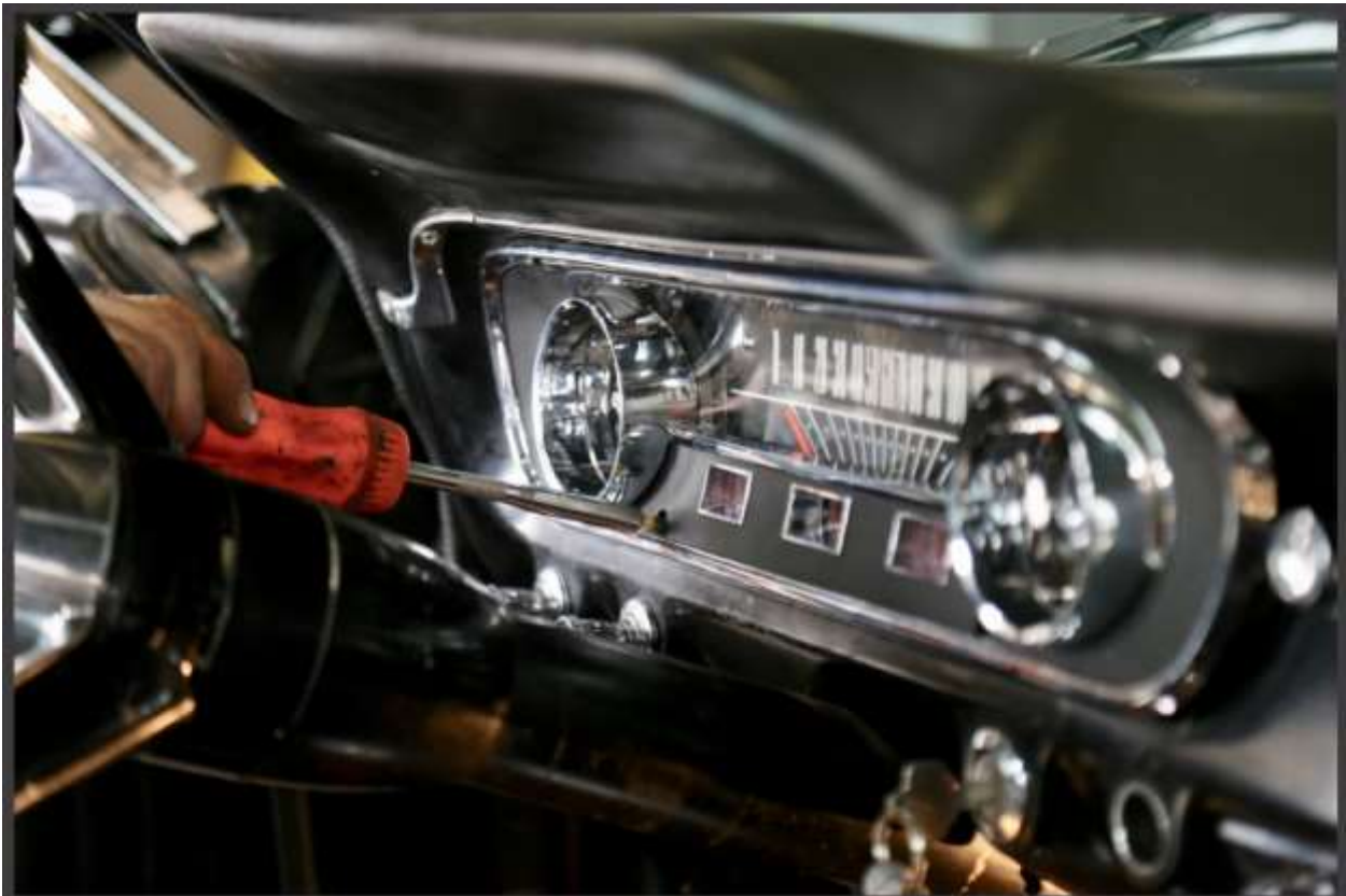
The instrument panel is secured with new hardware.
