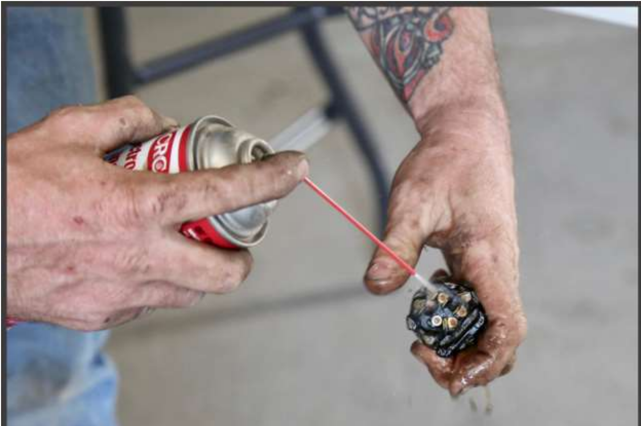
A couple of the switches were cleaned while others, such as the ignition and headlight, were replaced.
