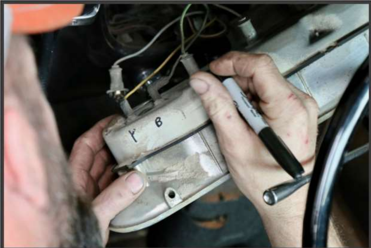
Using a permanent marker, Casey Barrett of Dakota Battery & Electric marks the wire colors and their position on the instrument panel housing. Note the worn and brittle condition of the wires and connectors.
