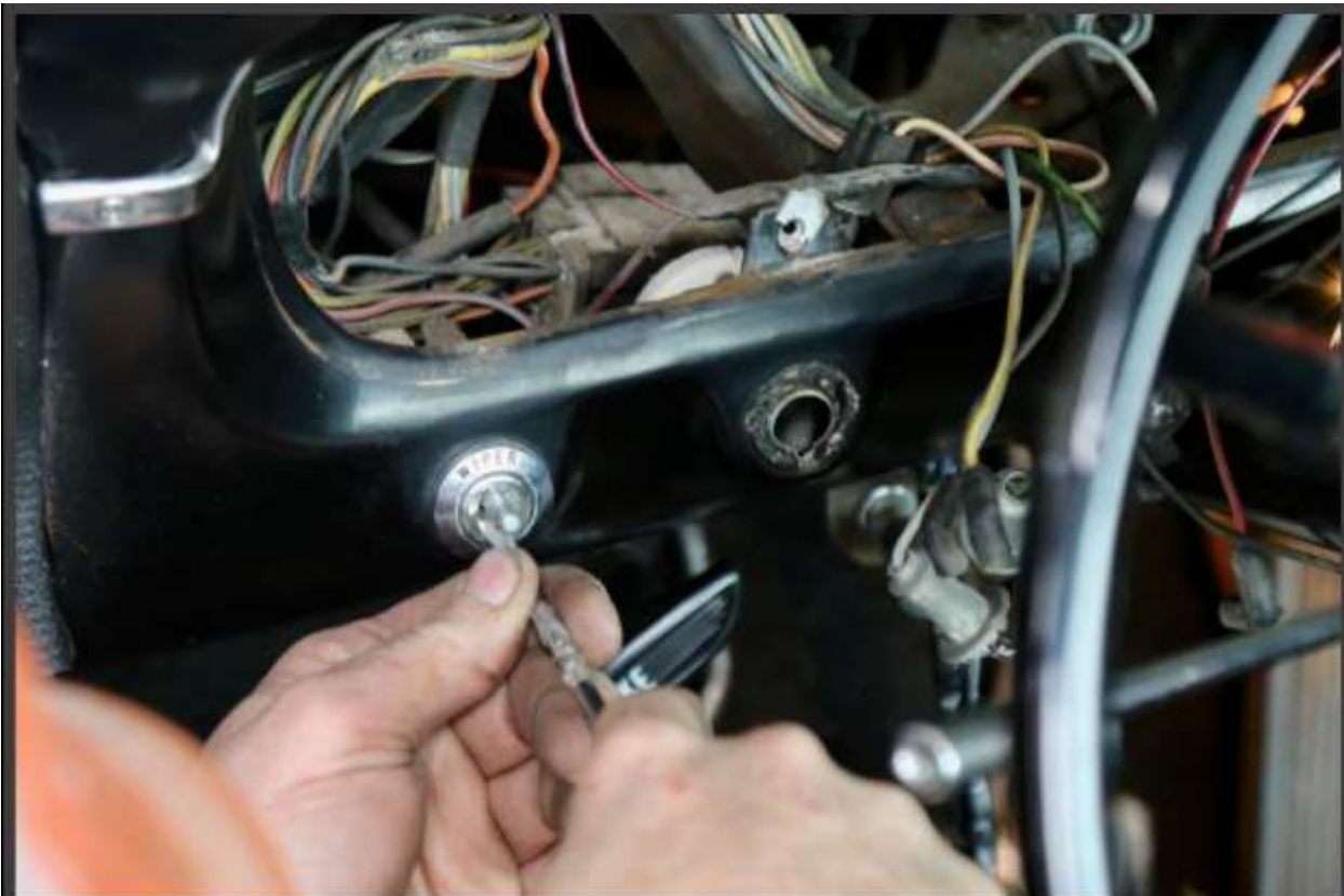
The disassembly continues by removing the wiper, headlight and other switches on the dash. Here, Barrett is using a small flathead screwdriver to turn and walk the internals out of the housing. Special tools are available to help remove or install some vintage switches.
