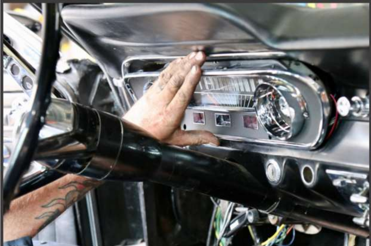
The gauge panel was positioned in the dash but not secured until a check of all the systems were conducted.
