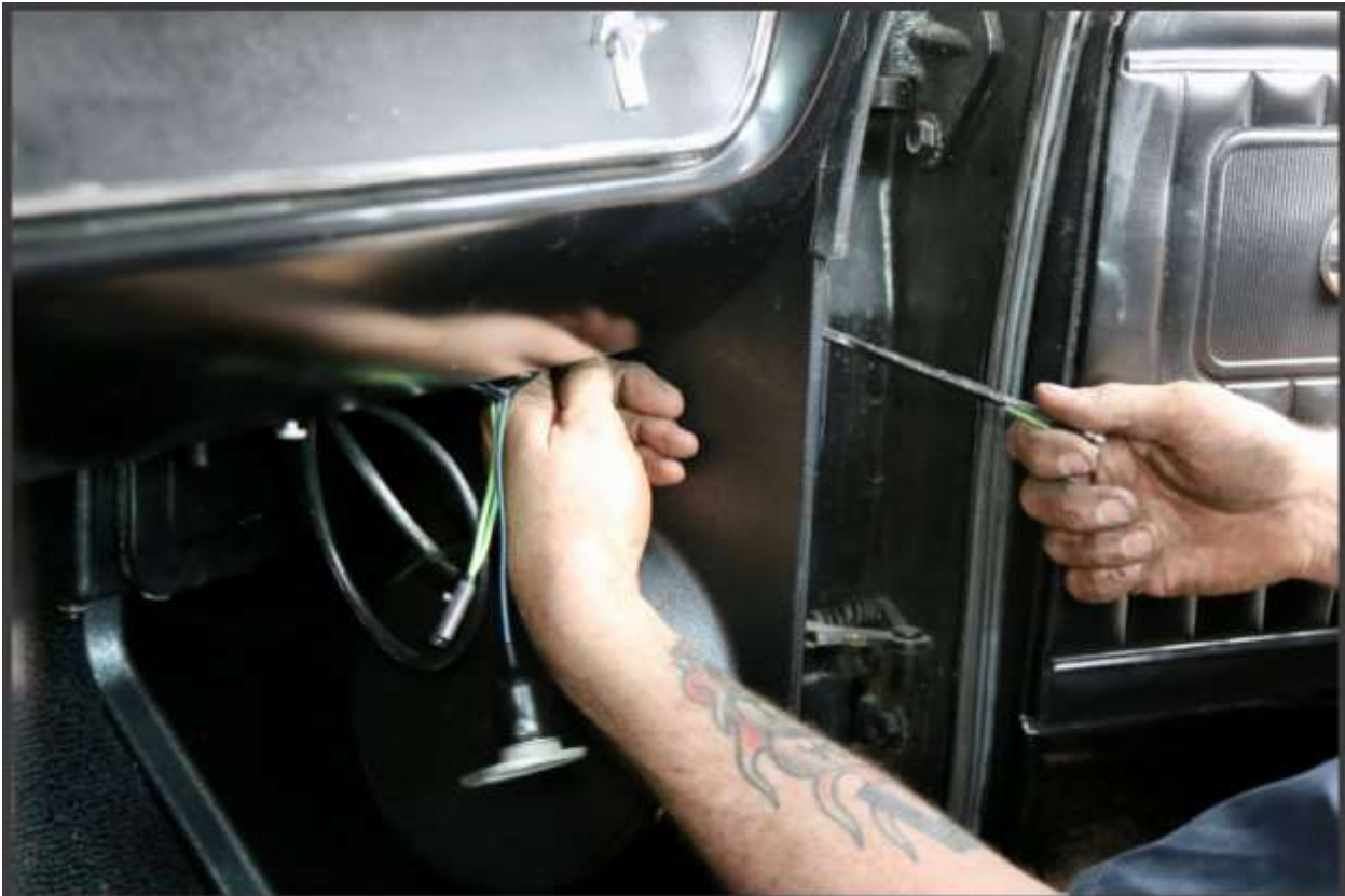
Under the right side of the dash, the speaker and door jamb dome light switch are connected, and the under dash courtesy light is also installed with a new bulb.
