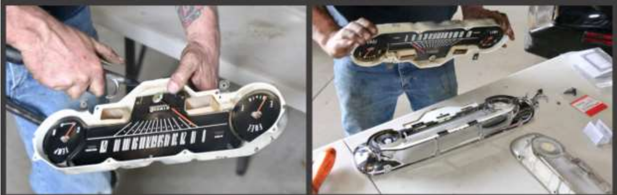
The instrument gauge is removed from the old bezel and dusted off with a light blast of compressed air before being fitted with a new bezel and lens.
