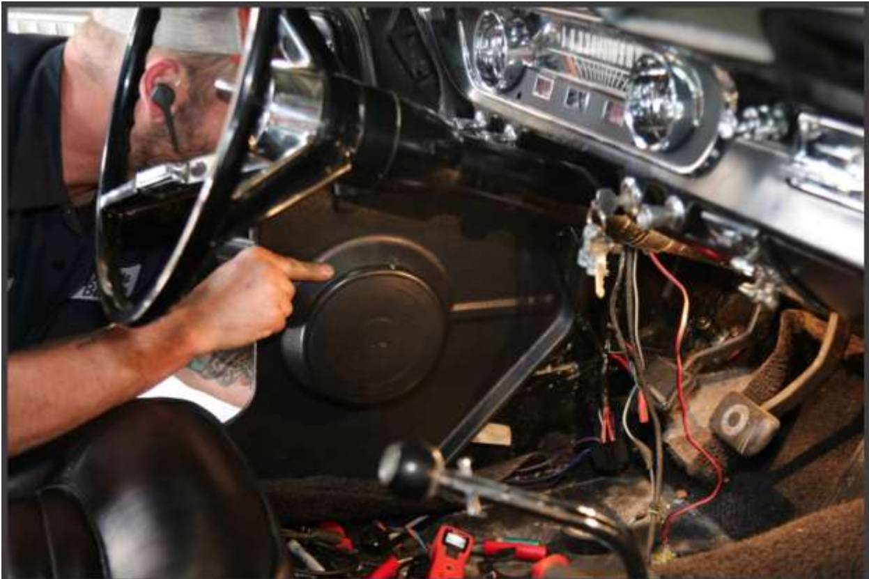
Scott Drake does provide a template to help mount the fuse panel, but it didn't work with the speakers. So, when the kick panel was replaced, the fuse panel was mounted to it near the stock location just above the speaker. Any loose wiring was wrapped with electrical tape and tucked up safely under the dash.
