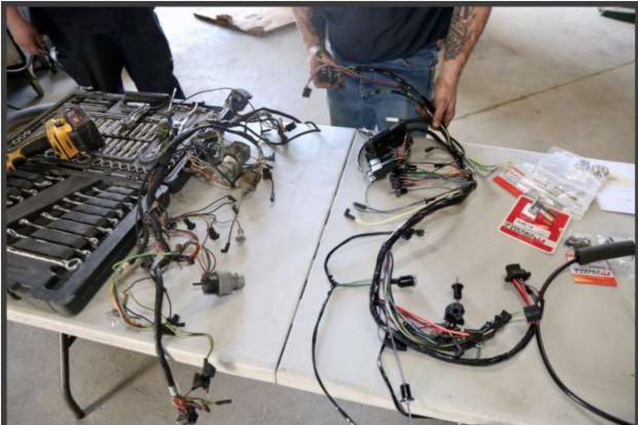
The old harness is compared to the Scott Drake harness on a large table. The type of connections and the colors of the wires were confirmed.
