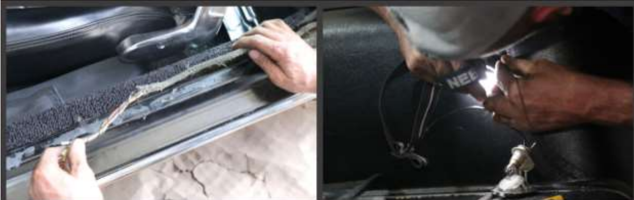
Removing the sill plate reveals the taillight harness. A "snake" needs to be attached to it, and then it's pulled from the trunk. Wiring for the two interior lamps on the fastback models also need to be snaked when removing the harness.
