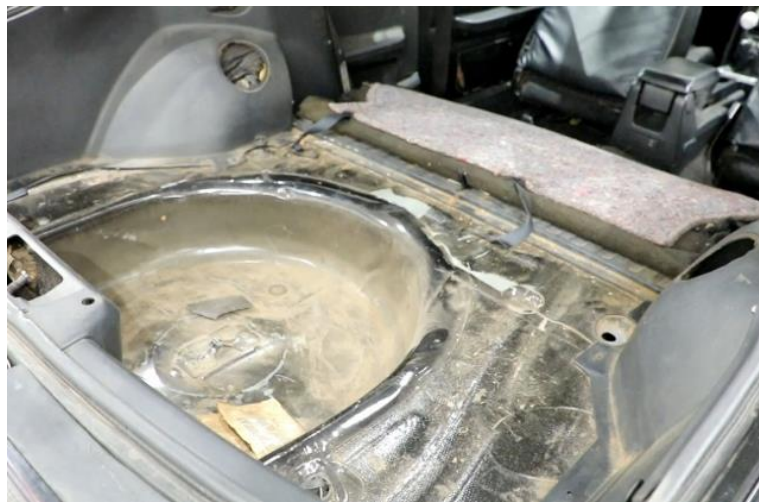
Figure 4 - Remove Trunk Carpet
