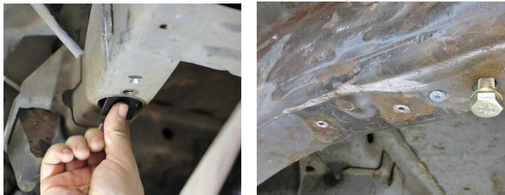
Figure 30 - Install Weld Nut Doubler Plates
