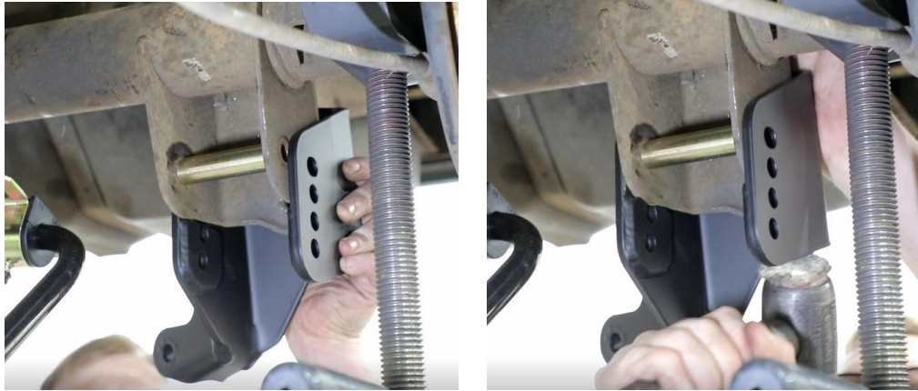
Figure 15 - Install Lower Coilover Bracket
