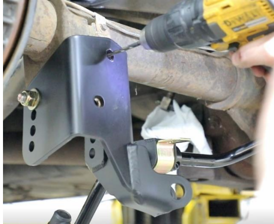
Figure 18 - Drill Axle Bracket Mounting Hole
