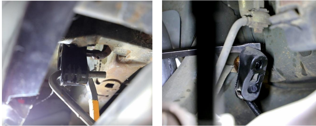
Figure 11 - Remove Exhaust from Hangers
