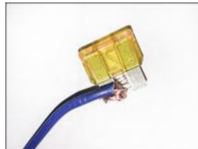
Wire Jammed Into a Fuse
