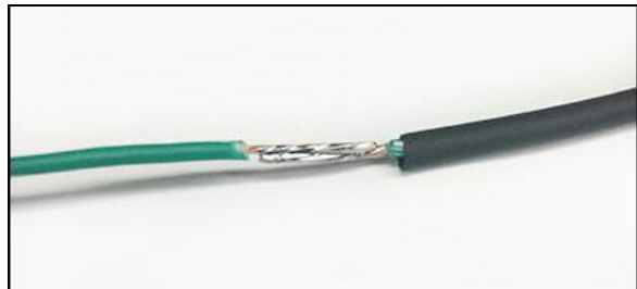
Soldered Connection w/ adhesive heat shrink
