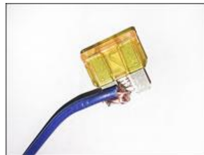
Wire Jammed Into a Fuse
