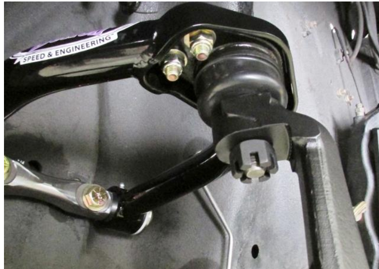
Figure 22 - Install Upper Ball Joint
