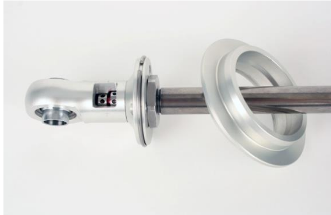
Figure 28 – Removing Lower Spring Seat
