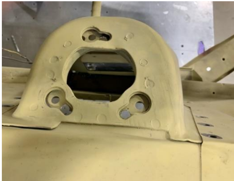
Figure 7 – Drill Strut Tower (Strut Tower Brace Not Pictured)
