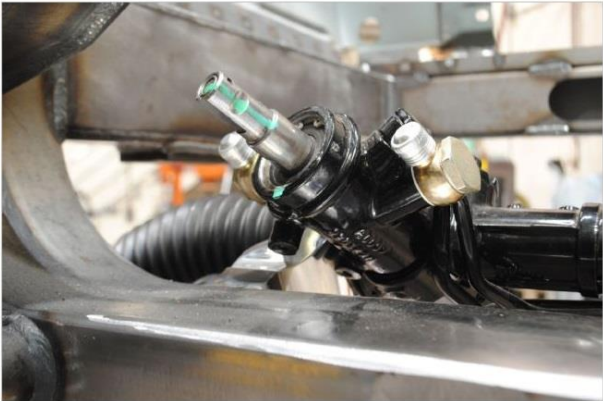
22. These two shots illustrate the adjustability in the steering rack mounts (and design).
