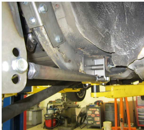
Figure 23. Start with Lower Link in center axle hole
