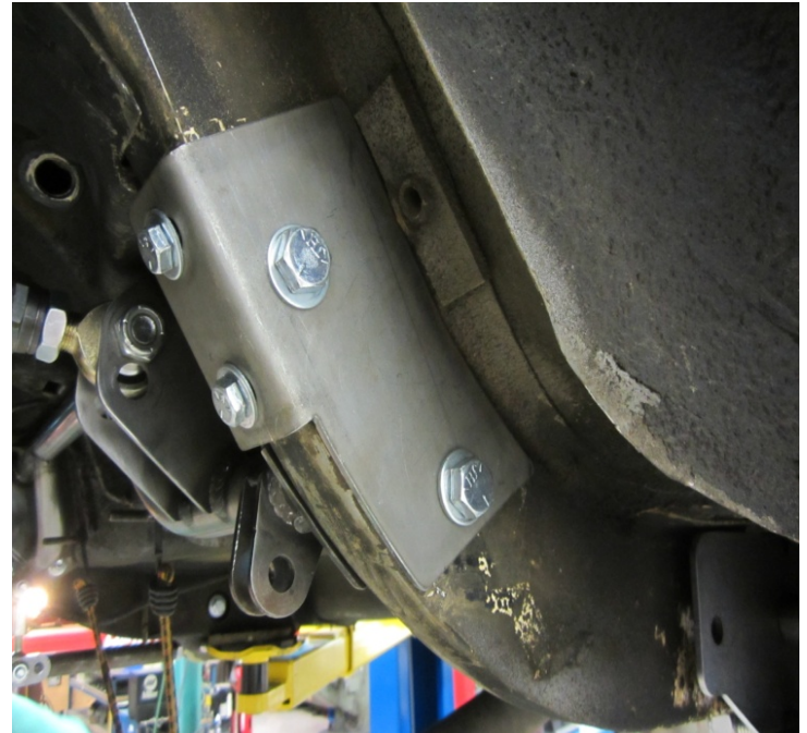
Figure 12. Tighten 1/2" bolts, then 3/8" bolts.
