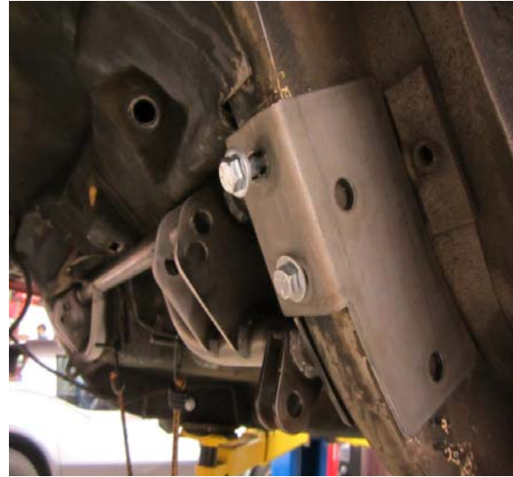
Figure 10. Install 3/8" bolts hand tight for now.
