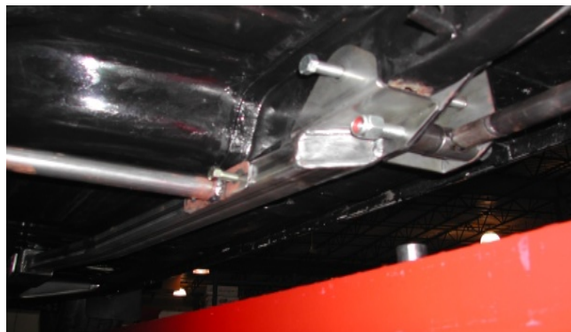
Figure 2. Subframe connector bolted to lower link bracket.
