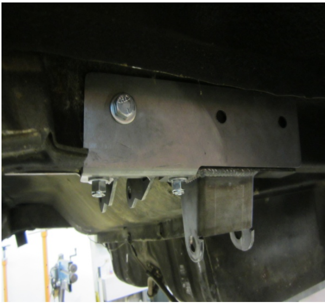
Figure 17. 1 (of 3) 1/2" bolts installed in driver side frame rail
