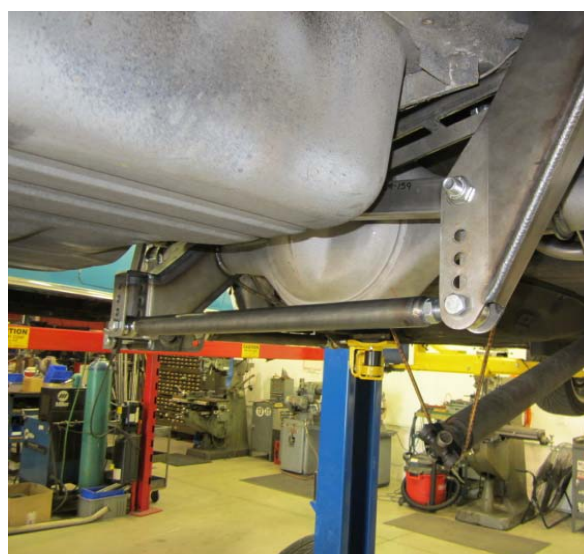
Figure 25. Panhard Bar: Start in bottom holes
