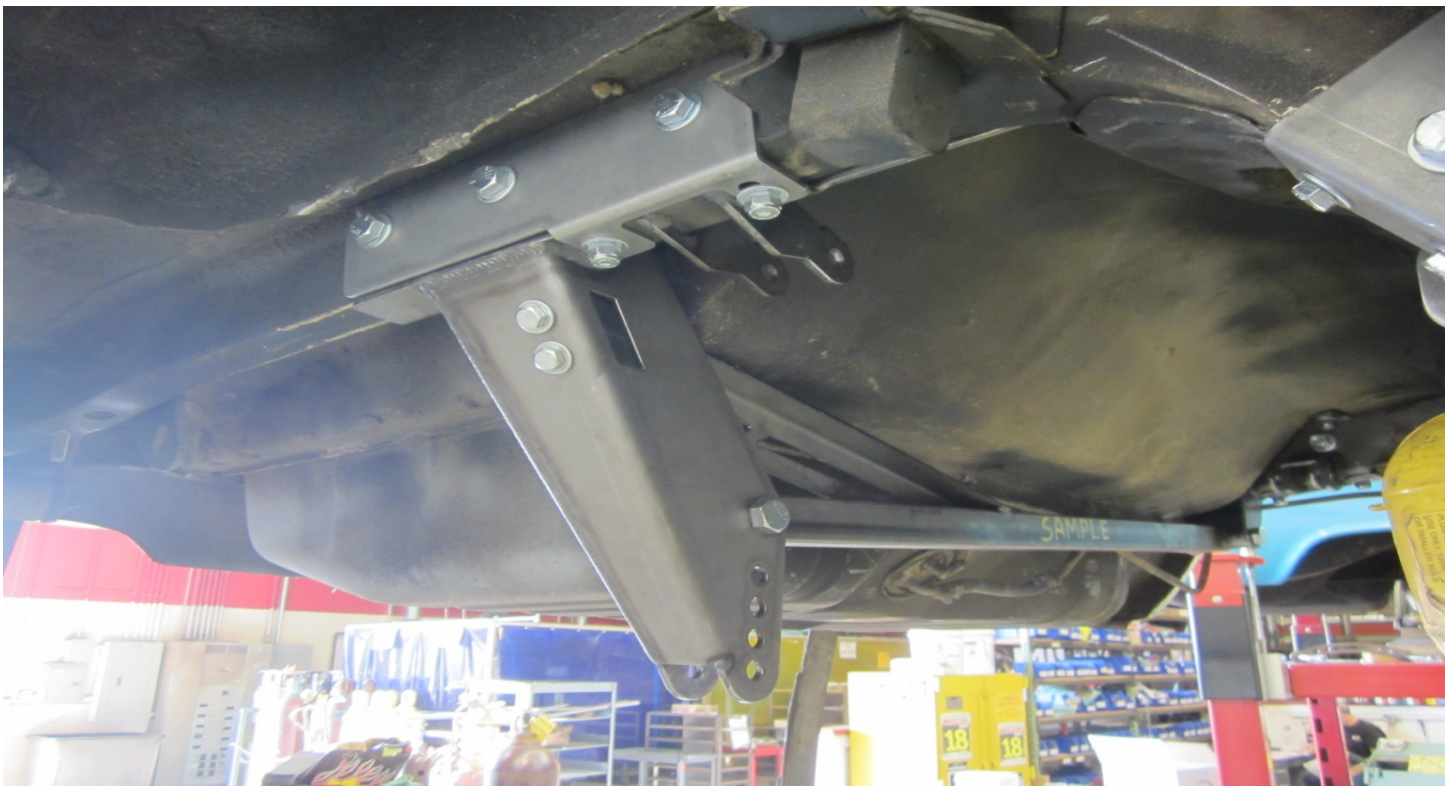
Figure 19. Assemble Panhard cross member hand tight.
