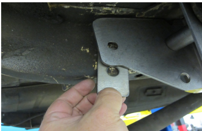
Figure 4. Use the same reinforcement plate on the inside frame rail.
