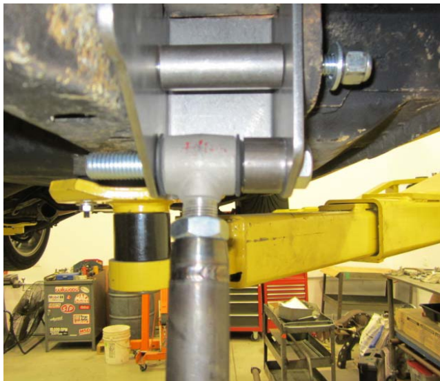
Figure 22. Passenger Side Lower Link: Spacer on the outside
