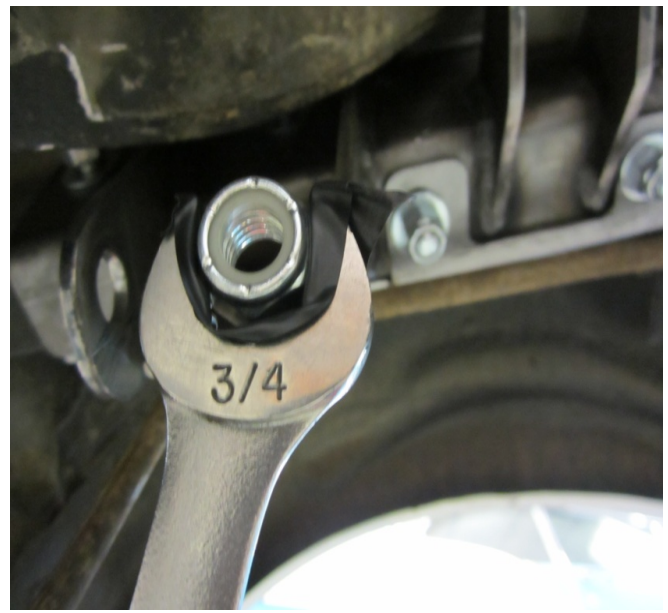
Figure 18. TIP: Use tape to hold the nut during install.
