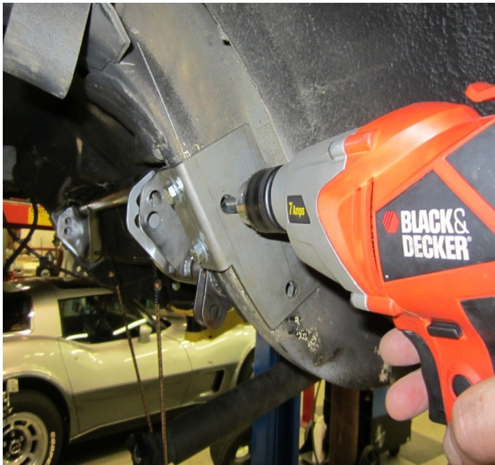
Figure 11. Drill frame rail, using brackets as a guide
