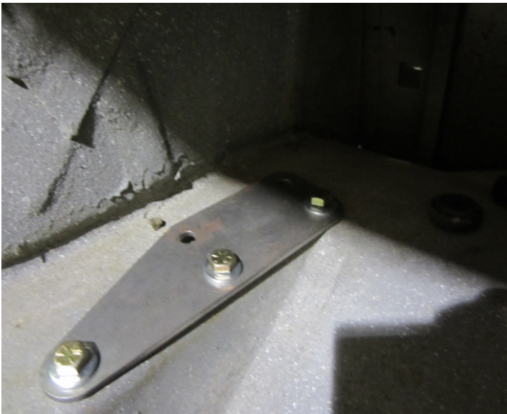
Figure 15. Driver Side Reinforcement Trunk Plate
