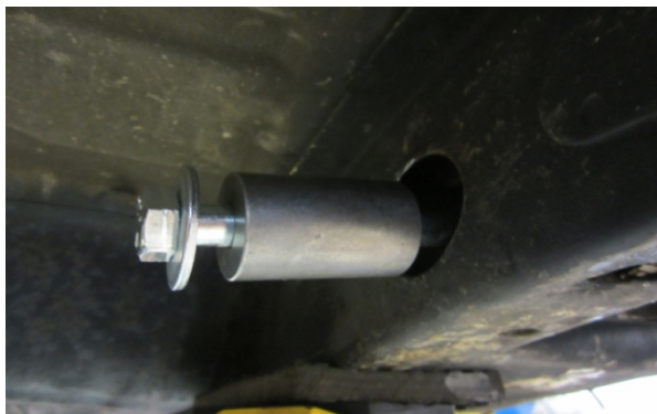
Figure 1. Spacer for 67-70 Mustangs only.
