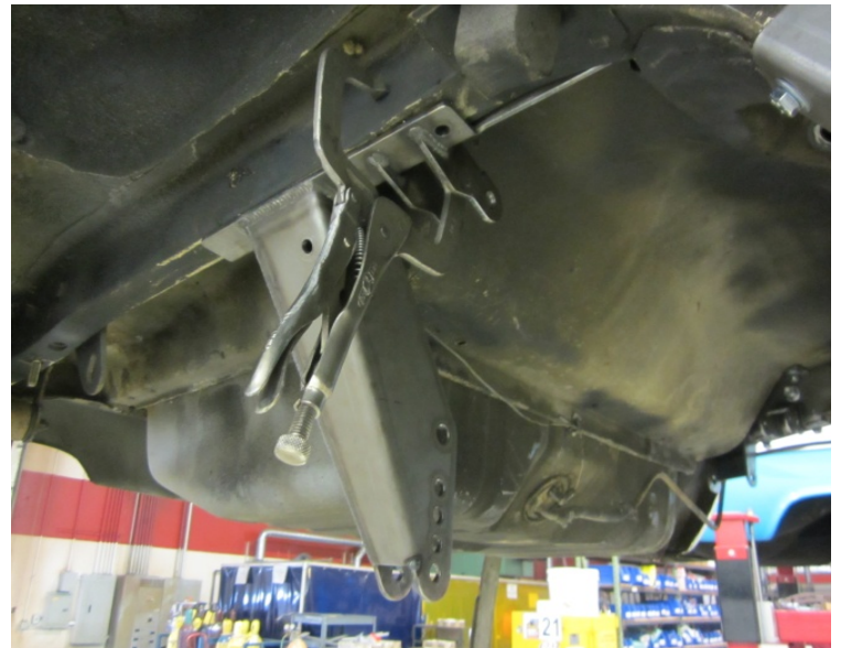
Figure 16. Use clamps to secure brackets while drilling
