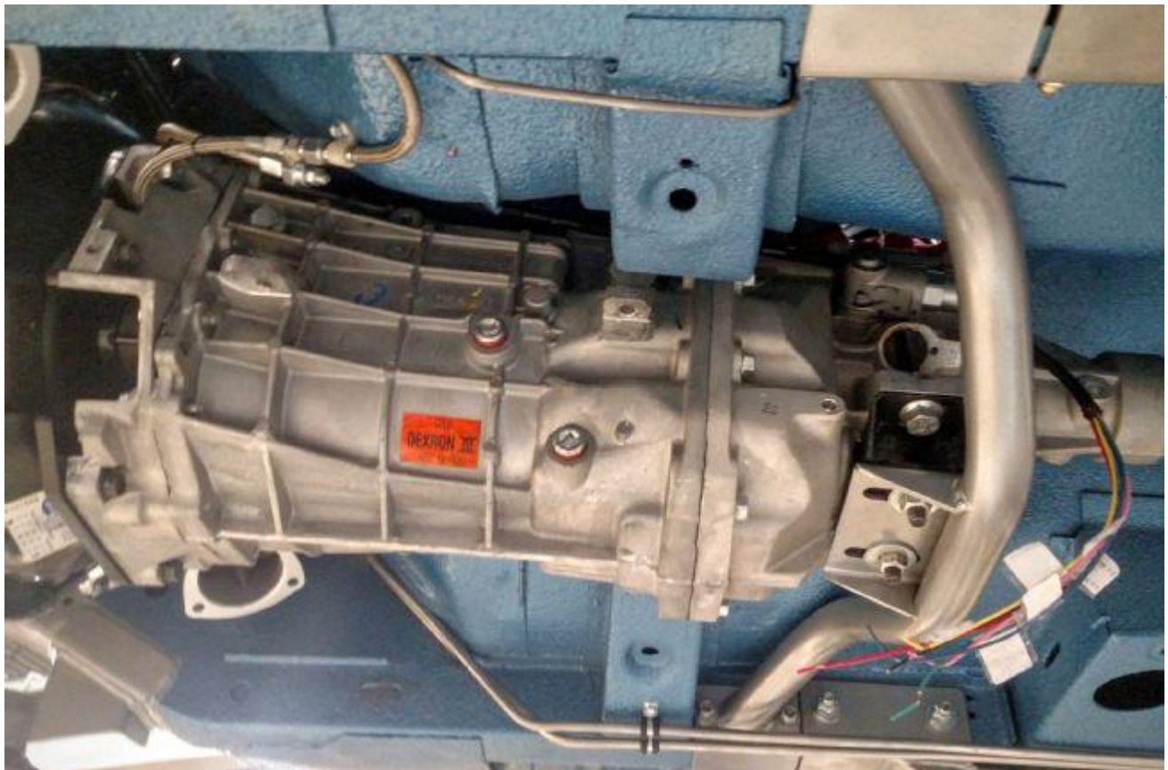
12. The transmission is a Tremec T-56 six-speed with a Quartermaster driveshaft (not yet installed) provided by Bruce Couture of Modern Driveline. "Bruce supplied the trans and everything from the flywheel to the input shaft," Leyshon says. "He possesses a wealth of knowledge and his help with the driveline was invaluable."
