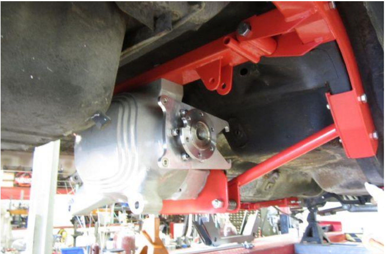
17. This is the passenger-side frame saddles, top crossmember, and IRS bare center section mounted during mockup. The center section (differential, ring-and-pinion, axles, and such) comes disassembled and must be put together by the end user.
