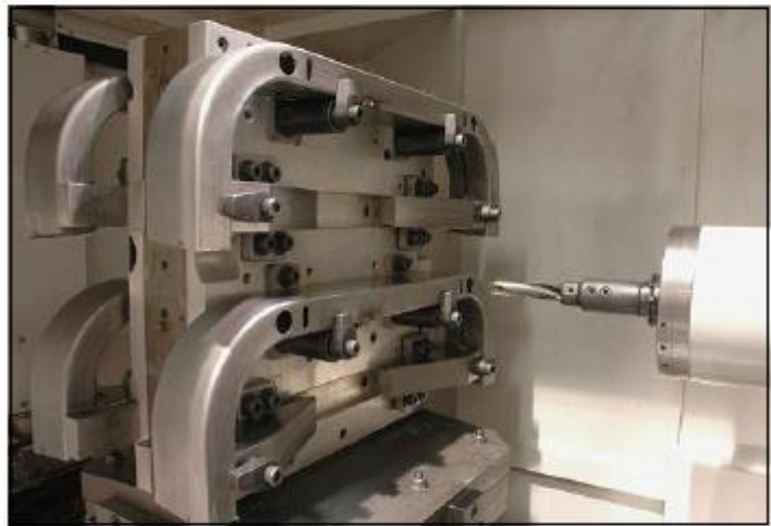
Locating features are machined into each crossmember to enable self-positioning of billet components.
